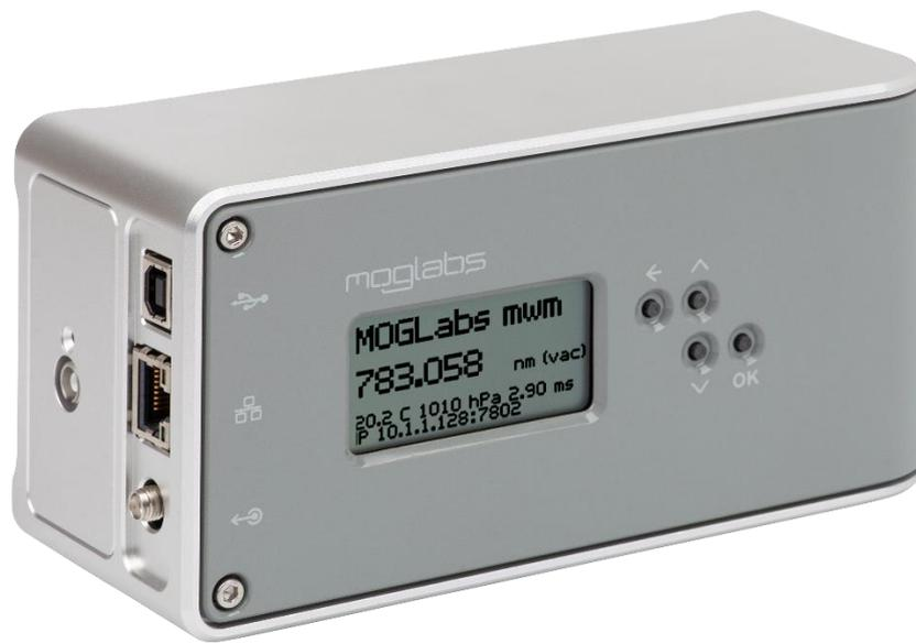
The MOGLabs Laser Wavemeter is a precision compact laser wavelength measurement device, and optical spectrum analyser, with on-unit display and ethernet/USB connectivity standard. Use it standalone or with the included Windows GUI software package.
